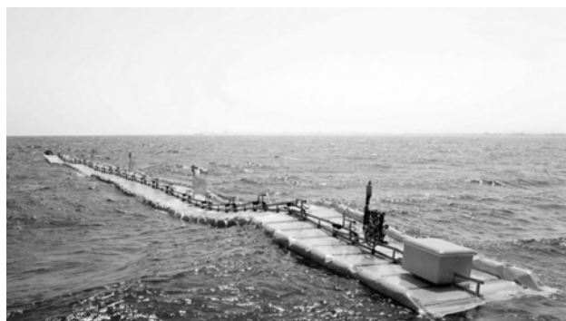
Fig. 4. Waveline Magnet floating generator [13]
