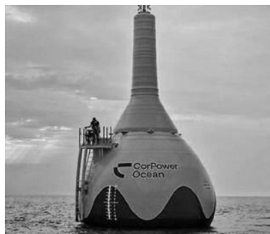
Fig. 3. CorPower floating generator [8]
